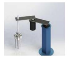
SCARA robot with a pneumatic gripper. Fingers made of Hyper-elastic Materials for the Poultry Industry. Applications include Palletization, pick & place and Gradation of eggs in weights.
